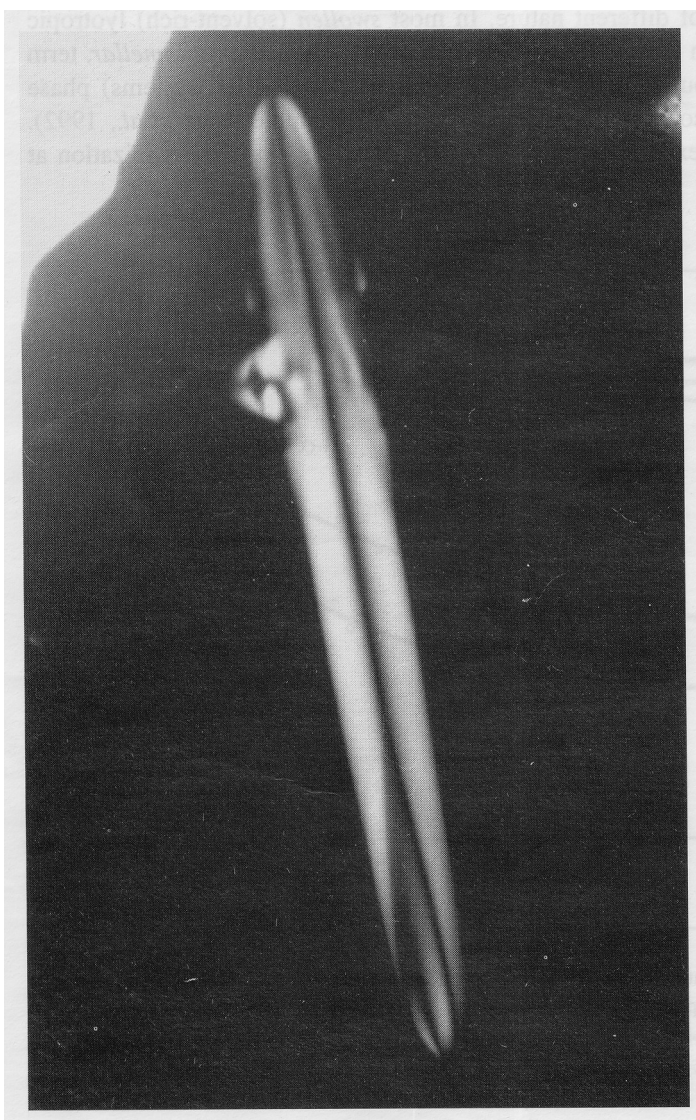
Fig. 2. – Nucleus (700 \mu\text{m} long) with a sword branch; the central body and the second branch are undeveloped. Same scale as in figure 3; polarizer almost parallel with the axis.
