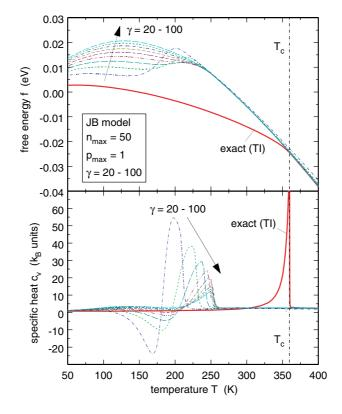
Fig. 5. Temperature evolution of f, expressed in eV (top plot), and  $c_V$ , expressed in units of  $k_B$  (bottom plot), for the JB model. The thick solid lines shows exact results obtained with the TI method, while the other lines show results obtained from Eqs. (3.14) and (3.15) with  $n_{\text{max}} = 50$ ,  $p_{\text{max}} = 1$ , and nine values of  $\gamma$  regularly spaced between  $\gamma = 20$  and  $\gamma = 100$ .
