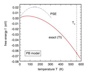
Fig. 1. Temperature evolution of the free energy per base pair f, expressed in eV, for the PB model. The solid line shows the exact result obtained from the TI equation, while the dashed line shows the result obtained from Eq. (3.10). The vertical dot-dashed line indicates the correct critical temperature  $T_c$  determined from the TI equation.
