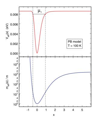
Fig. 6. Plots of  $V_{\text{eff}}(x)$ , expressed in eV (top plot), and  $m_{\text{eff}}(x)/m$  (bottom plot), for the PB model at T = 100 K.  $V_{\text{eff}}(x)$  and  $m_{\text{eff}}(x)$  are defined in Eq. (5.2). The horizontal segment in the top plot shows the energy  $\mu_1$  of the lowest eigenstate of the generalized PSE in Eq. (5.1).
