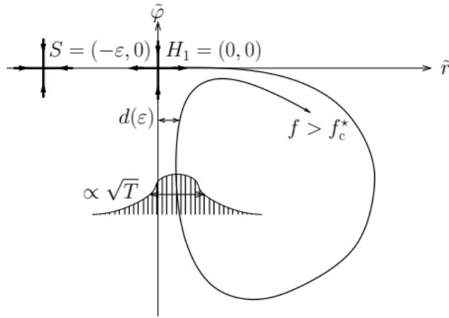
$$\text{escape time} \sim \underbrace{\exp\left(\frac{\epsilon^3}{T}\right)}_{\text{Arrhenius}} \underbrace{\exp\left(-\frac{A}{T}d(\epsilon)^2\right)}_{\text{Trapping probability}}$$
