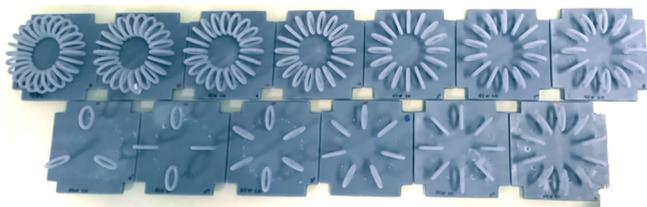
FIG. 2. Different fabrications of toroidal cages with different number of tori from  $N = 3$  to  $N = 24$ , placed along a circle of radius  $R_T = 32.5$  mm.
